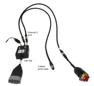
7. Connect the other end of the 1-Meter Patch cable (102730) to either the Secondary EXP-100 or the DCM-300 Adaptor (100906).
