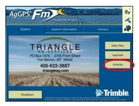
Highlight Variable Rate & Section Control and check that it reads 'Unlocked'.
