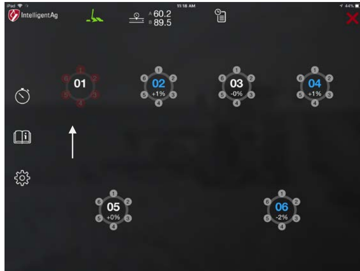
Figure 18: Blockage screen showing a manifold not seeding due to section control
