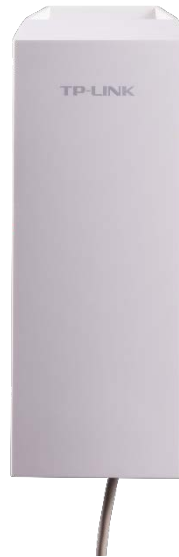
Figure 21: Wireless Blockage and Flow Monitor access point
