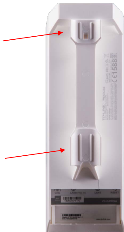
Figure 24: Apply the gaskets to the feet of the access point
